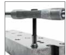
Setting the extractor with a tap wrench
