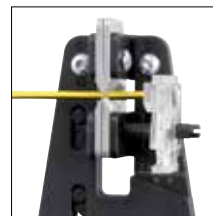
Cable is accurately positioned at length stop
