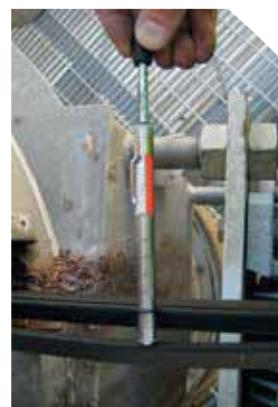
Using the tension tester ensures that correct tension is maintained and is repeatable. This will yield not only a longer service life but a predictable one, enabling scheduled replacement rather than breakdown replacement.
