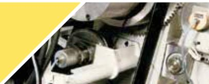
This compact and strong belt with nominal top width from 3mm to 11mm transmits more power and allows high speed ratios.
